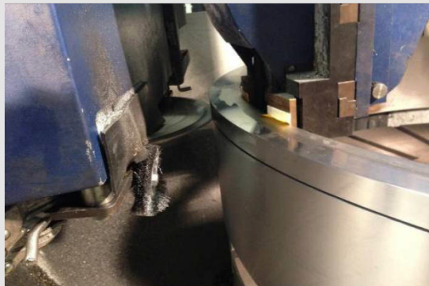
Process of cutting with 3 mm slitting width
