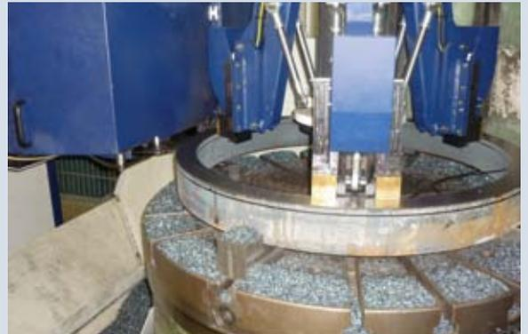
▲ Three clamping jaws hold the ring as it rotates, making for a clean cut.
