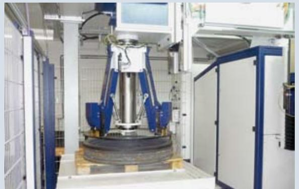
▲ The handling unit sets the rings aside, ready for further processing.
